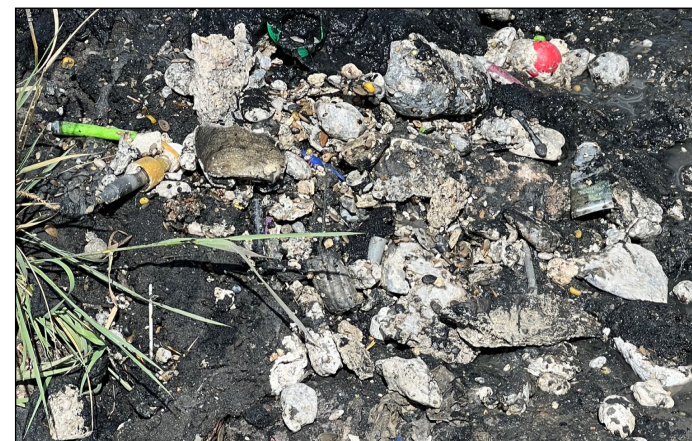
FMCV workers along with Moencopi Water/Wastewater take a short lunch break Pictures below and across show debris in sewer lines causing backup.
