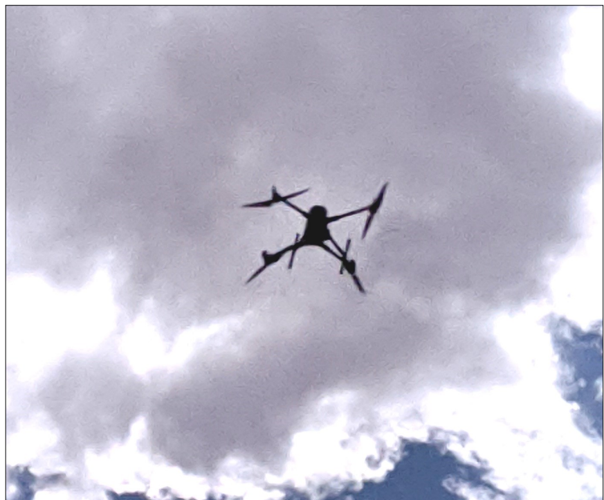
Drone launched to take photos for survey points of flood area
